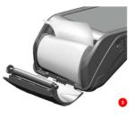
Hold the terminal securely in one hand. With the other hand, and by using two fingers, lift the printer cover release as shown. Fully open the printer cover and remove the old roll of paper.
