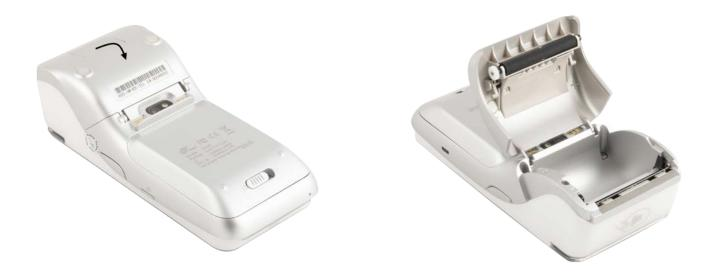
Once open, place the receipt roll provided into the open compartment with the receipt paper extending from underneath the roll leaving at least 1cm exposed and close the cover.
