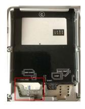
Insert the SIM card in the slot as shown below and left;
