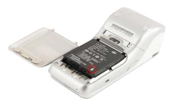
Lift the battery at the bottom (by the white arrow) and remove it from the terminal.
